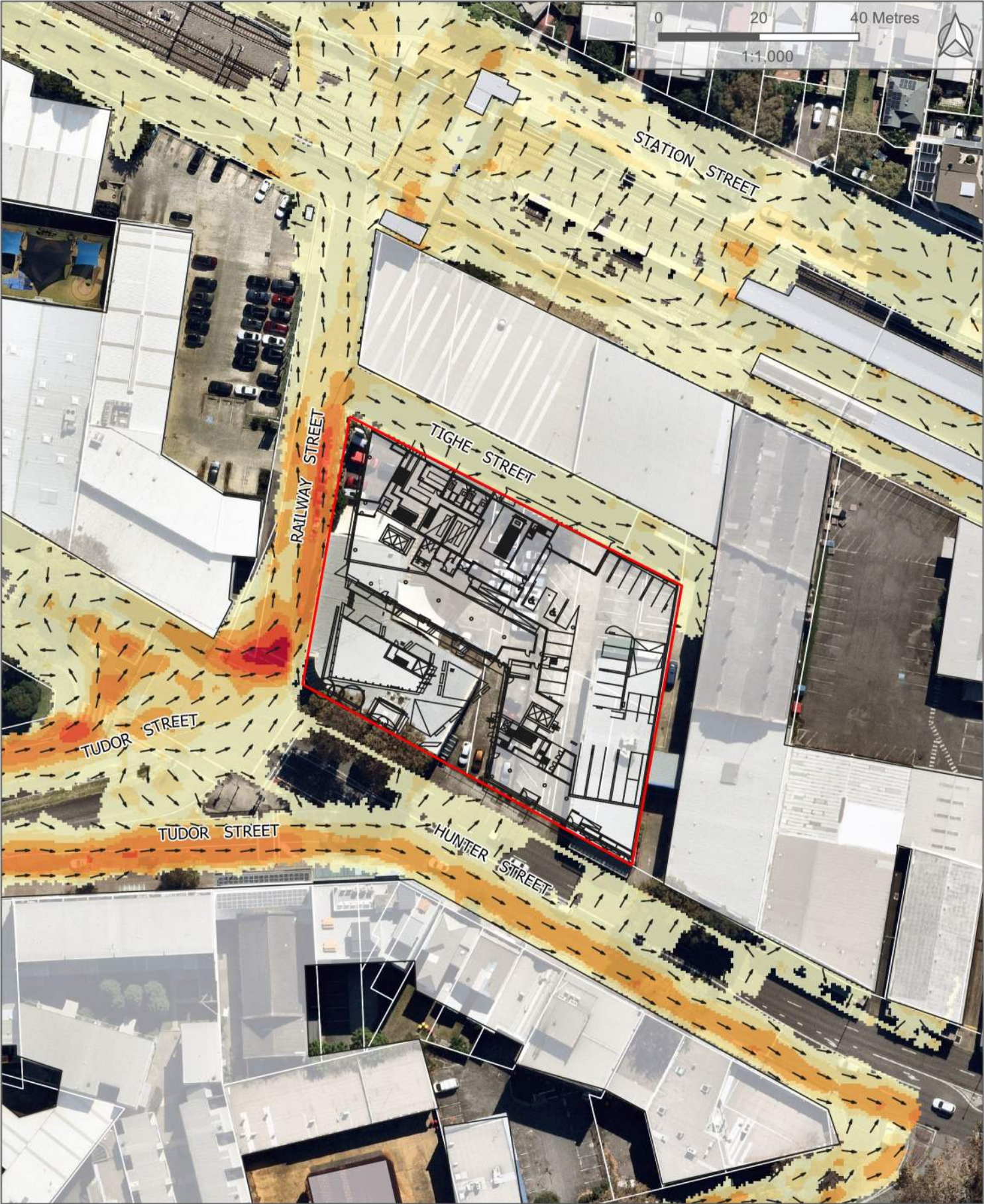
Figure C5 Developed Case 1% AEP Flood Velocity and Vectors
